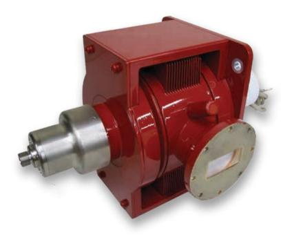
A magnetron is a high power microwave oscillator in which the potential energy of an electron cloud near the cathode is converted into RF energy in a series of cavity resonators. The VMC3136 magnetron delivers high peak and average RF power for use in medical or industrial applications.
